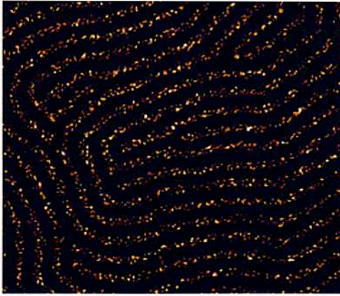
Transmission electron micrograph of self-assembled hybrid nanostructure (organic polymer and metals).
